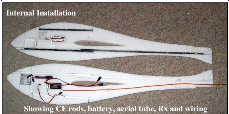
Showing servos, switch, snakes and hatches for battery and Rx
